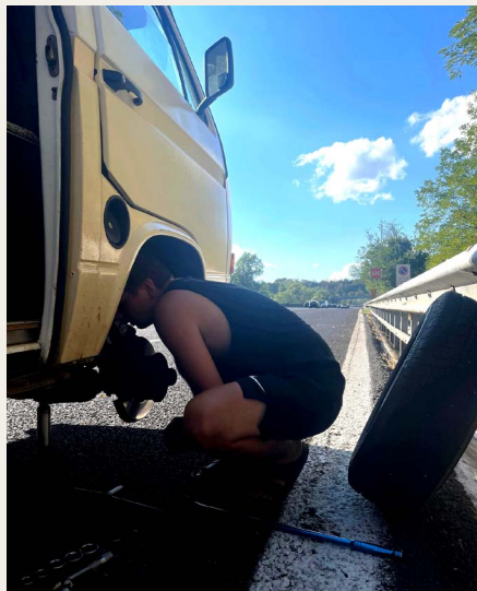
Reparation af CV-led
